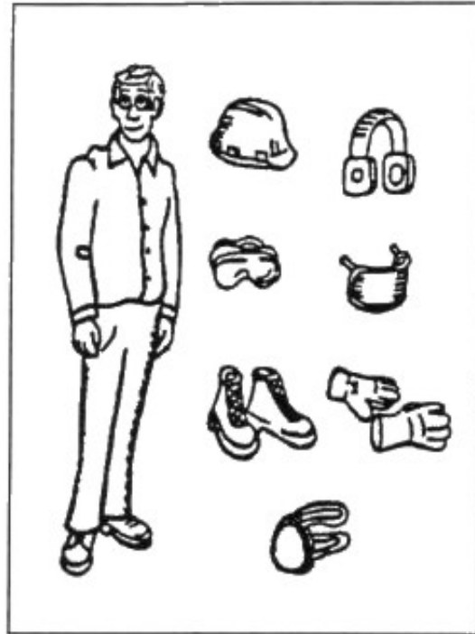
Figure 1. Sturdy clothing, gloves, safety hat, eye and ear protection, and safety shoes are necessary for safe operation of the cut-off saw
